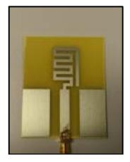
Figure 4: Antenna prototype of dual-band monopole antenna
