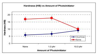
Fig. 6. Hardness of Samples at Different Amount of Photoinitiator.
