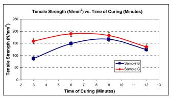
Fig. 5. Tensile strength of samples at different curing time exposure
