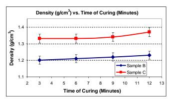
Fig. 3. Density of samples at various curing time exposure
