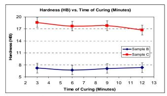
Fig. 7. Hardness of Samples at Different Curing Time
