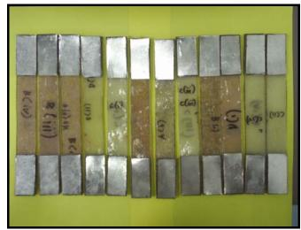
Fig. 1. Specimen for tensile test ASTM D3039
