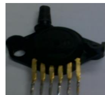
Figure 3 MPX4250AP CASE 867B-04 with pin configurations
