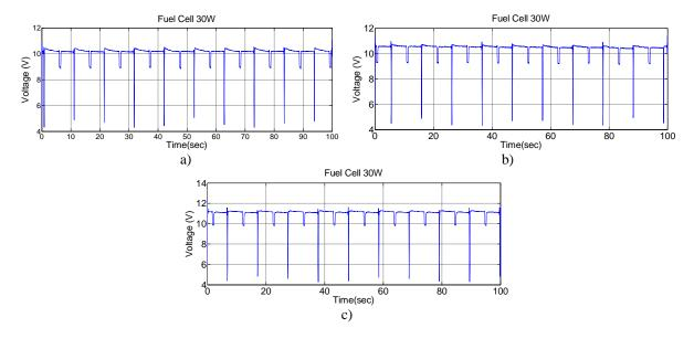
**Fig. 2:** Performance voltage (V) of 30W PEMFC with different of hydrogen (H<sub>2</sub>) pressure at anode side: a) 0.1 bar H<sub>2</sub> pressure b) 0.3 bar H<sub>2</sub> pressure c) 0.5 bar H<sub>2</sub> pressure.
