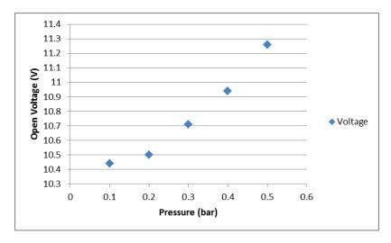
Fig. 3: Effect of pressure towards the PEMFC voltage at open voltage condition.
