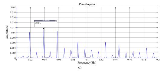
**Fig. 4:** Periodogram of 30W PEMFC with different of hydrogen (H<sub>2</sub>) pressure at anode side: a) 0.1 bar H<sub>2</sub>pressure b) 0.3 bar H<sub>2</sub> pressure c) 0.5 bar H<sub>2</sub>pressure
