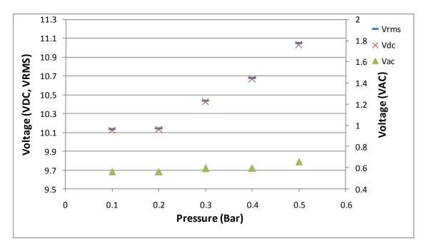
Fig. 6: Periodogram data of  $V_{DC}$ ,  $V_{RMS}$ , and  $V_{AC}$  at various pressures.
