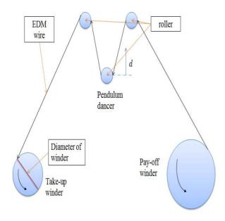
Fig. 1. Schematic diagram of rewinding machine
