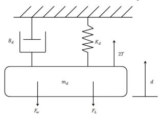
Fig. 5. Mechanical model of dancer
