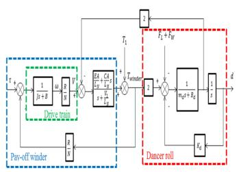
Fig. 8. The complete system of the wire winding system
