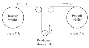
Fig. 4. Sketch of wire winder system
