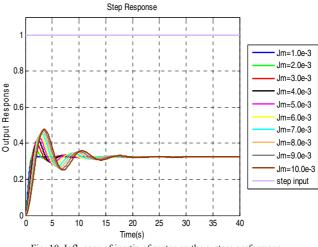
Fig. 10. Influence of inertia of motor on the system performane
