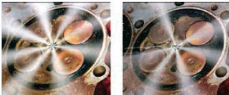
Figure 2.1 : Close up of new (left) and worn (right) fuel injector nozzles.
