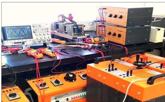
**Figure-5.** Experimental setup for series R-L load test.
