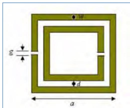
Figure 1.2 Geometries of the ring under analysis.
