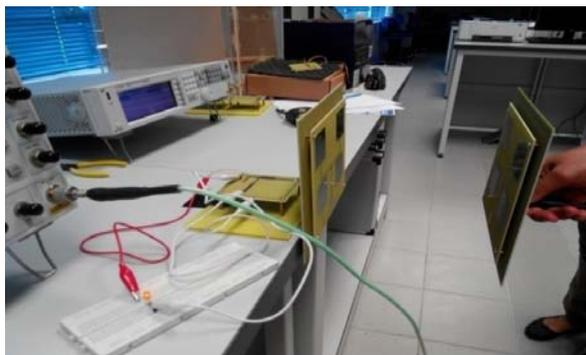
Figure-8. The measurement setup for integrated antenna with rectifier circuit experiment.
