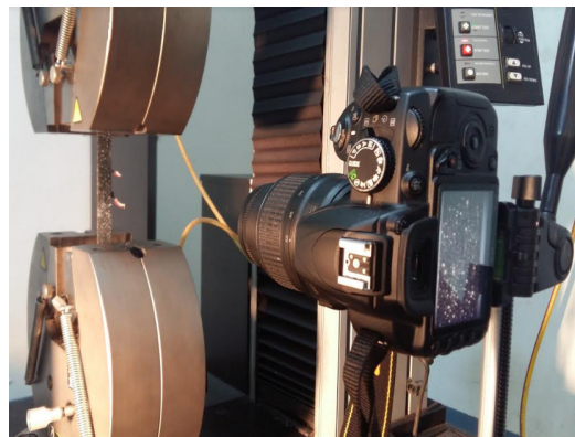
Figure 2: Image with speckle on the surface of object acquired by camera
