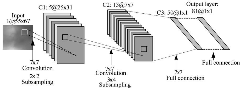
Figure-16. Best model for VeCAD-UTM finger-vein database (5-13-50).
