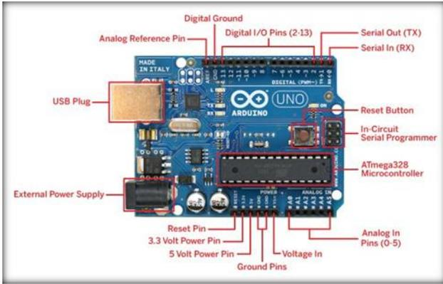
Fig. 10. Basic Configuration of Arduino UNO microcontroller
