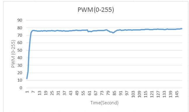
Fig. 23. Output for  $K_p=0.010$ ,  $K_i=0.3$ ,  $K_d=0$
