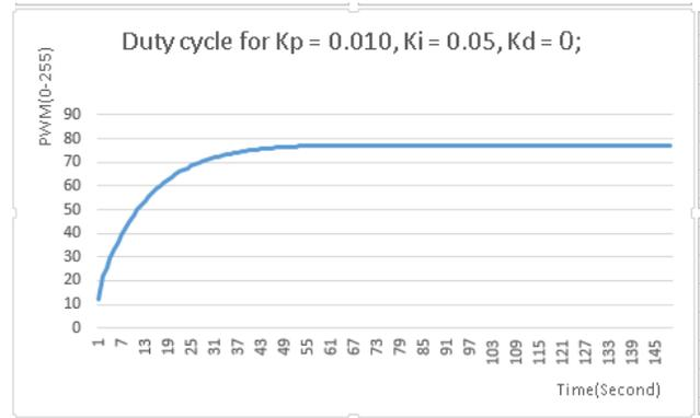
Fig. 19. Output for  $K_p=0.010$  ,  $K_i=0.05$  ,  $K_d=0$
