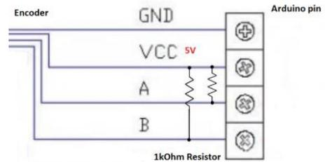
Fig. 8. Rotary encoder connection to Arduino
