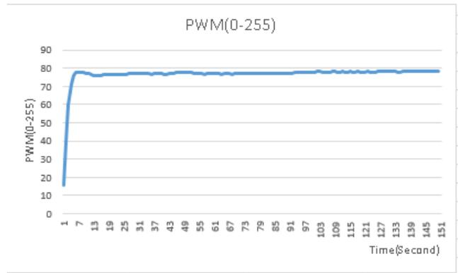
Fig. 25. Output for  $K_p=0.010$ ,  $K_i=0.3$ ,  $K_d=0.01$
