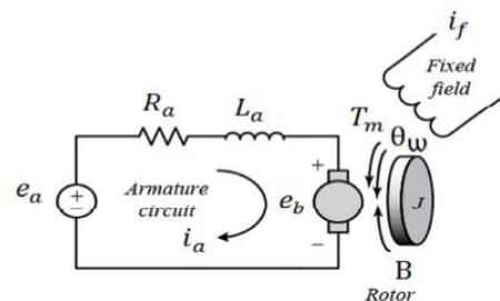
Fig. 1. Equivalent circuit for DC motor
