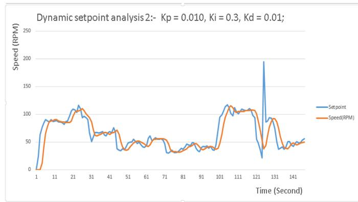
Fig. 32. Dynamic se tpoint analysis 2,  $K_p=0.010$  ,  $K_i=0.3$  ,  $K_d=0.01$
