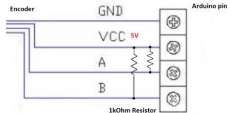
Fig. 8. Rotary encoder connection to Arduino
