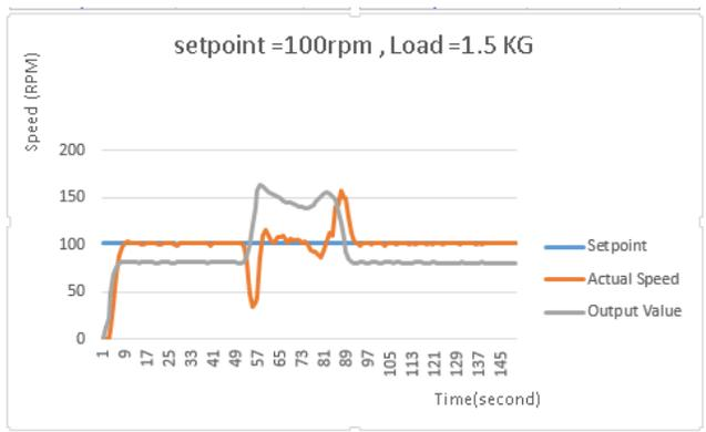
Fig. 28. Closed loop test with load disturbance 1.5 kg
