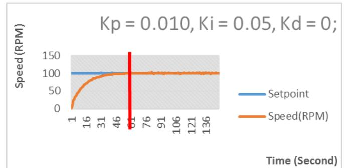
Fig. 18. PID tuning  $K_p=0.010$  ,  $K_i=0.05$  and  $K_d=0$
