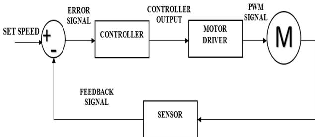
Fig. 3. Closed loop system block diagram.
