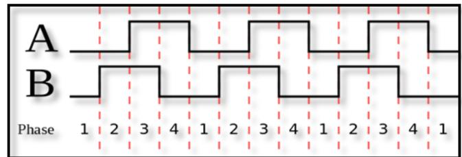
Fig. 9. Two output from rotary encoder represent two square wave in rotary encoder
