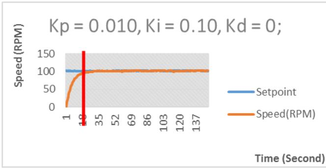
Fig. 20. PID tuning  $K_p=0.010$  ,  $K_i=0.10$  and  $K_d=0$
