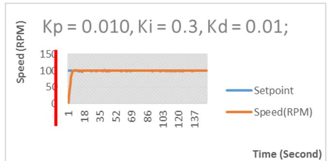
Fig. 24. PID tuning  $K_p=0.010$  ,  $K_i=0.3$  and  $K_d=0.01$
