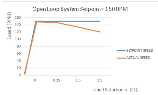
Fig. 13. Load disturbance test with setpoint 150 rpm
