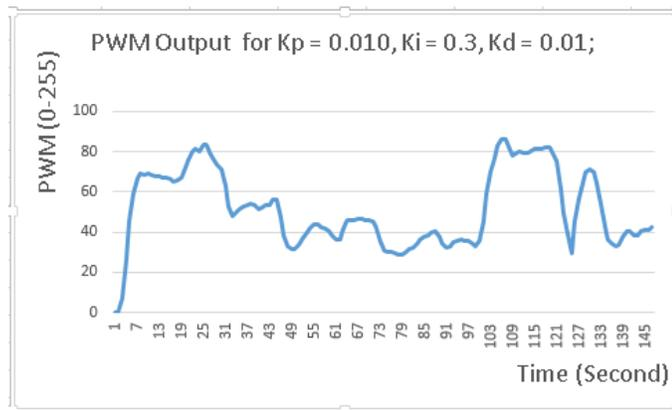
Fig. 33. Output value for  $K_p = 0.010$  ,  $K_i=0.3$  ,  $K_d=0.01$
