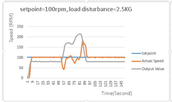
Fig. 29. Closed loop test with load disturbance 2.5 kg
