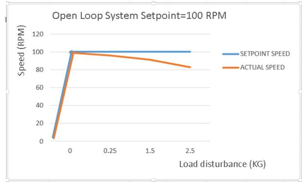
Fig. 12. Load disturbance test with setpoint 100 rpm
