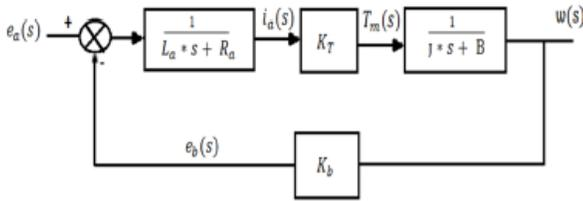
Fig. 2. DC motor armature control system block diagram
