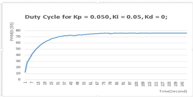
Fig. 15. Output for  $K_p=0.050$  ,  $K_i=0.05$  ,  $K_d=0$
