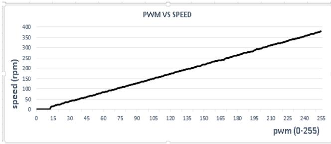
Fig. 11. PWM Input vs Speed of DC Motor (Open Loop)
