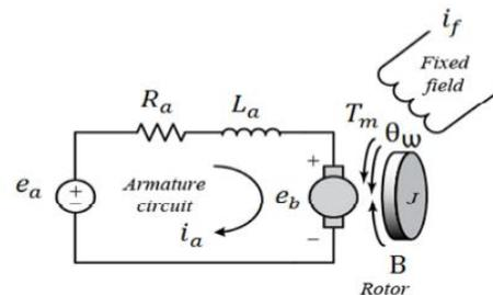
Fig. 1. Equivalent circuit for DC motor
