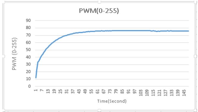
Fig. 17. Output for  $K_p=0.10$  ,  $K_i=0.05$  ,  $K_d=0$
