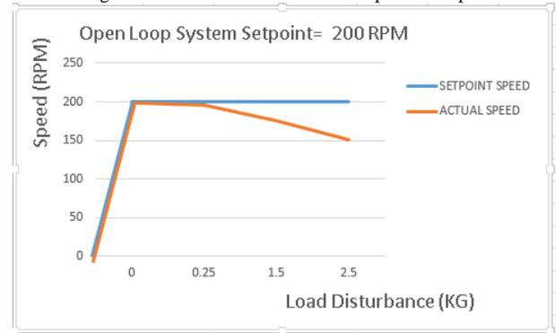
Fig. 14. Test load disturbance with setpoint 200 rpm
