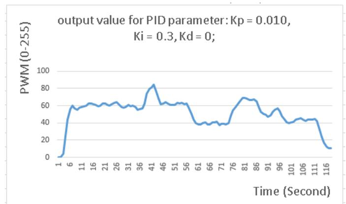
Fig. 31. Output value for  $K_p = 0.010, K_i=0.3, K_d=0$
