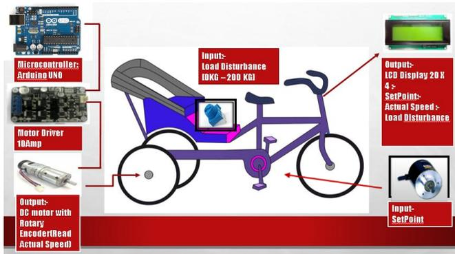
Fig. 5. Conceptual design of trishaw
