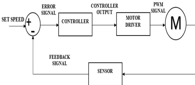
Fig. 3. Closed loop system block diagram.
