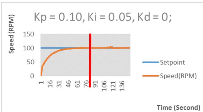
Fig. 16. PID tuning  $K_p=0.10$  ,  $K_i=0.05$  and  $K_d=0$
