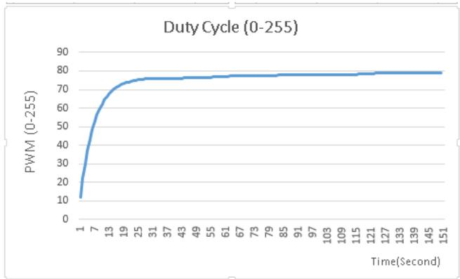
Fig. 21. Output for  $K_p=0.010$ ,  $K_i=0.1$ ,  $K_d=0$
