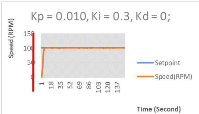
Fig. 22. PID tuning  $K_p=0.010$  ,  $K_i=0.3$  and  $K_d=0$
