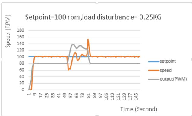
Fig. 27. Closed loop test with load disturbance 0.25 kg
