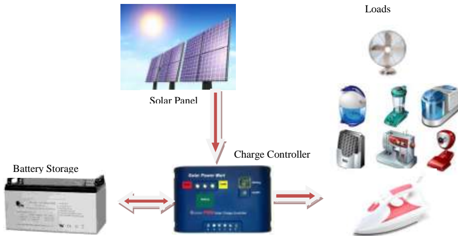
Figure 1. Conventional Method of Photovoltaic System Connected to Load
