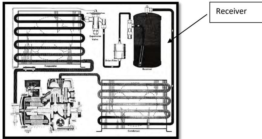
**Figure 2.1** Refrigeration system with a receiver (Gajdhar 2015).
