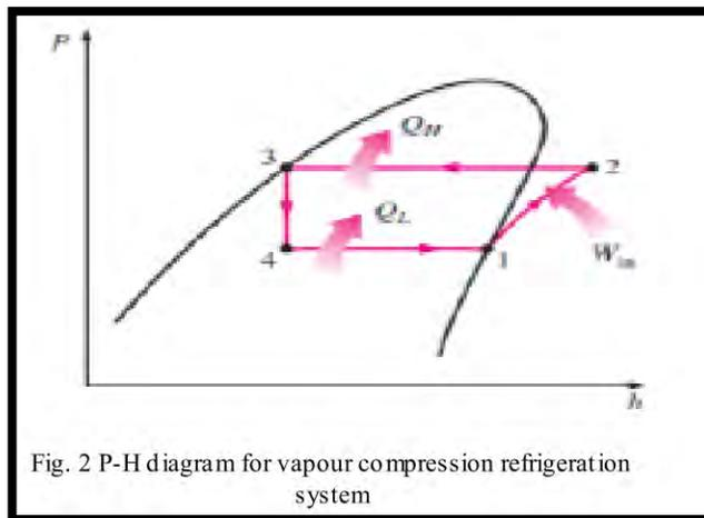
Fig. 2 P-H diagram for vapour compression refrigeration system
