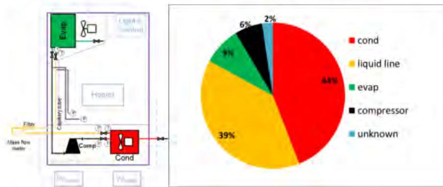
From table 2.1, the refrigerant charge in the condenser and liquid line where the receiver is installed has the highest charge than other components in the system which are 44% and 39%. The liquid refrigerant should be stored in receiver before discharging to the expansion valve in saturated liquid refrigerant.
