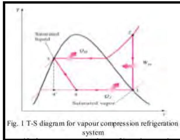
Fig. 1 T-S diagram for vapour compression refrigeration system
