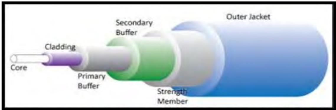
Figure 2.3: Basic structure of an optical fiber
