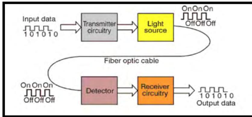
Figure 2.1 Basic fiber optic communication system
