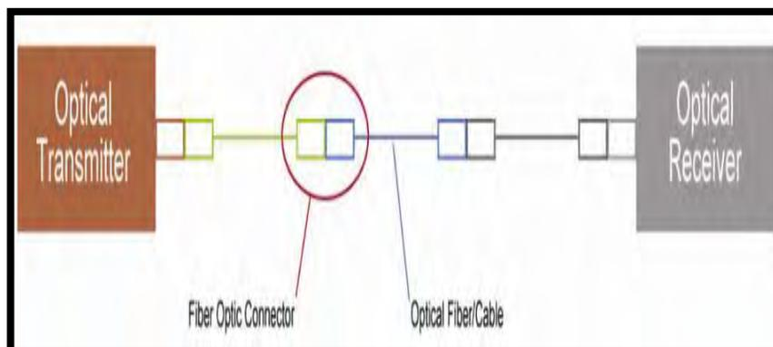
Figure 2.2: Simple Fiber Optic Link
