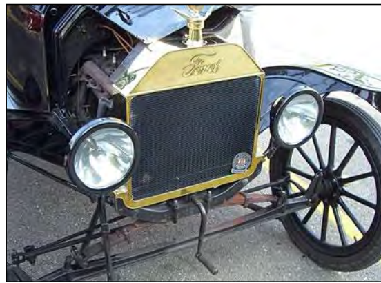
Figure 2.1: Hand Cranks Starter on Ford Model T (Larry, 2009)
