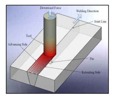
Figure 1.1: Schematic diagram of FSW process (Cavaliere et. al., 2006).
