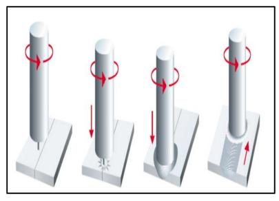
Figure 1.2: Stages of the friction stir welding (Shtrikman, 2008).
