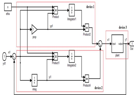
Figure 3 Adaptive PI tuning state block diagram
