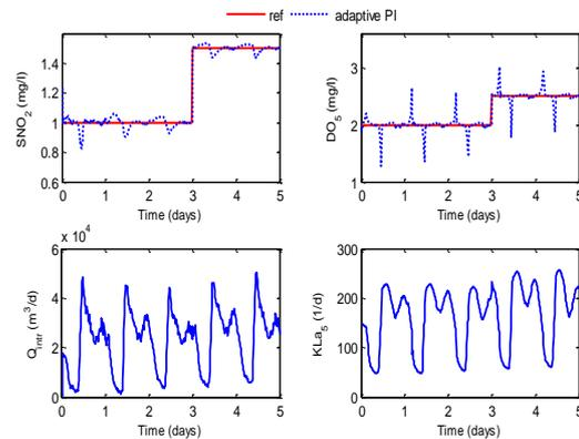
Figure 5 Tracking control performance under dry weather
