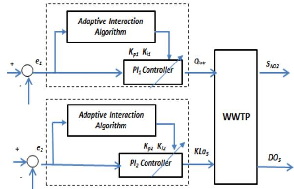
Figure 4 The implementation of adaptive decentralized PI
