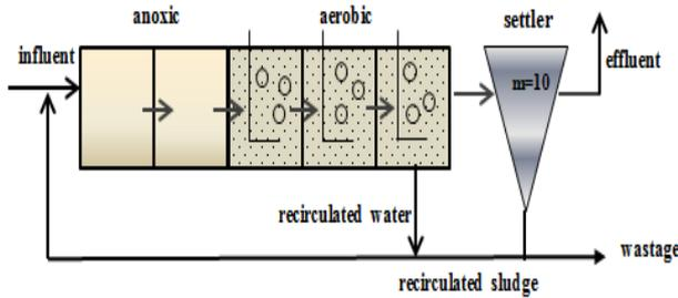
Figure 1 The plant layout of the BSM1
