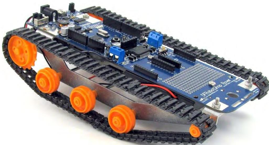
**Figure 1.1 Track system robot.**
