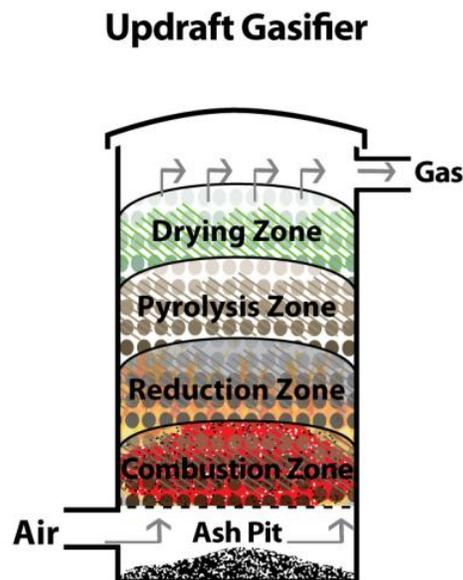
Figure 2.1: Four Zone Process in Updarft-Gasifier
