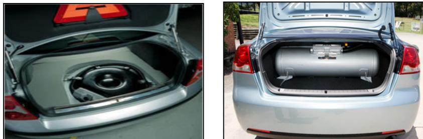
Fig 2.2.2 LPG Tank in boot (From left Donut and Cylindrical shape)
