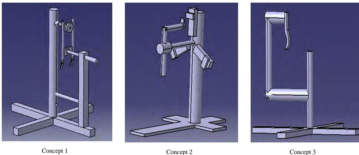
Fig. 4 Concept designs of motorcycle tire dismantling tool
