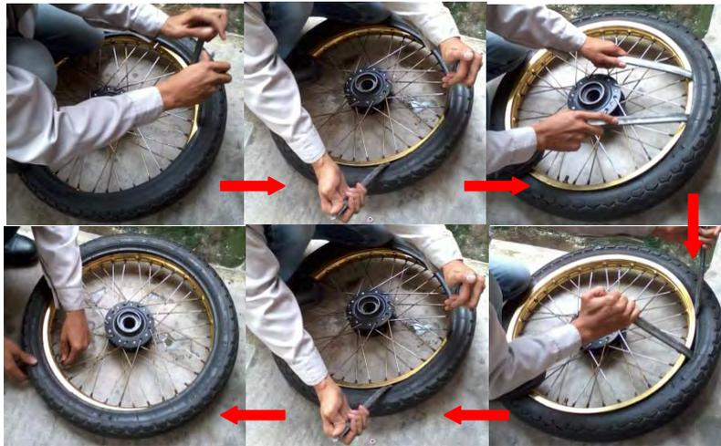
Fig. 2 Current practice of the motorcycle tire dismounting process
