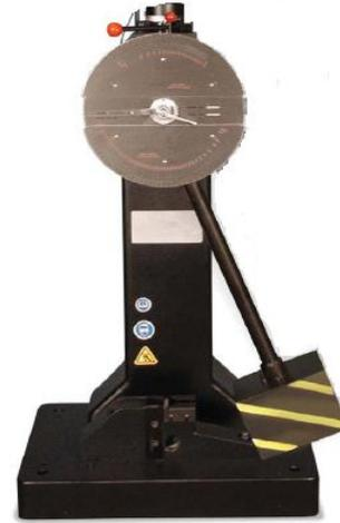
Figure 3 Pendulum impact apparatus for the experiment
