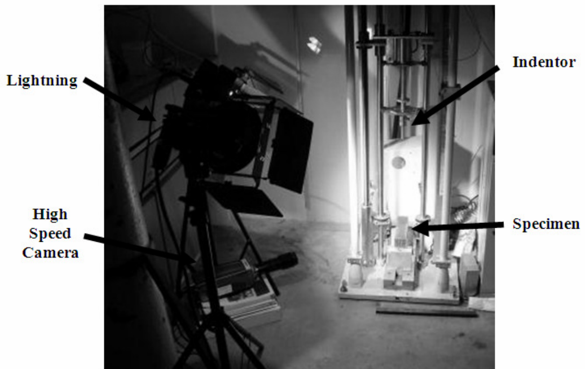
Fig. 4. High-speed camera set up.
