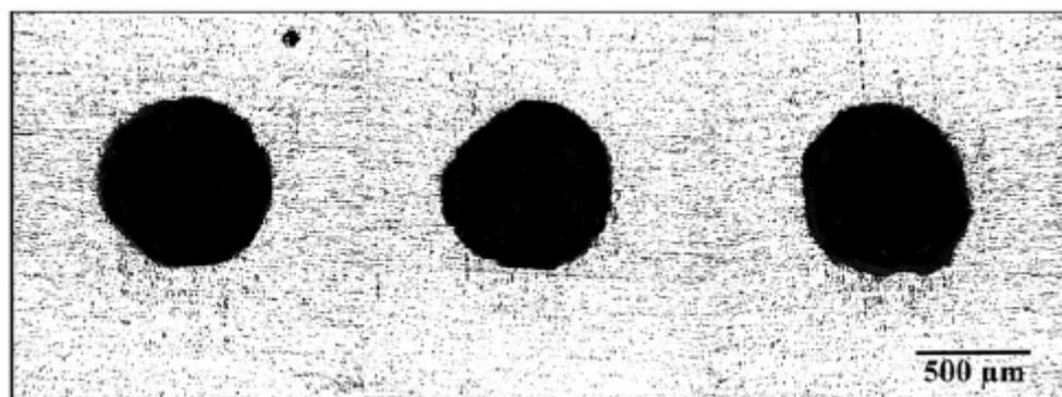
*Figure 1.1: Variation of entrance geometry of laser percussion drilled holes under the same operating parameter setting [2].*
