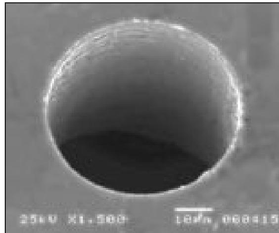
Figure 2.7: 150 micron diameter hole in silicon [16]
