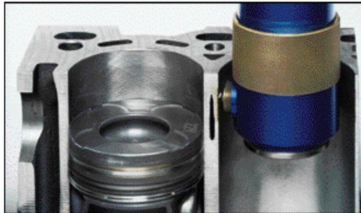
*Figure 1.2: Laser texturing of engine cylinder walls [3].*
