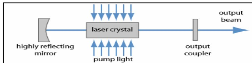
Figure 2.4: Setup of a simple optically pumped laser [9].
