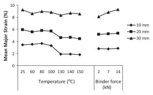
Fig. 3. Main-factor effects at point A for mean major strain at different depths.
