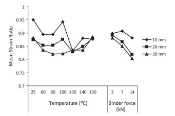
Fig. 4. Main-factor effects at point A for mean strain ratios at different depths.
