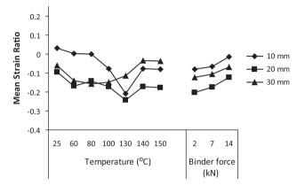
Fig. 6. Main factor effects at point B for mean strain ratios at different depths.
