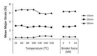
Fig. 7. Main factor effects at point C for mean major strain at different depths.
