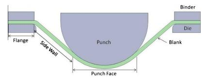
Fig. 1. Location terminology on the blank during forming [16].
