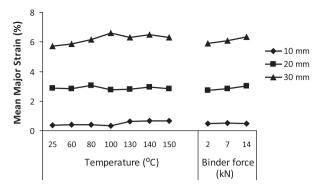
Fig. 5. Main factor effects at point B for mean major strain at different depths.
