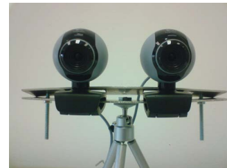
Figure 1. Horizontally aligned of stereo camera.
