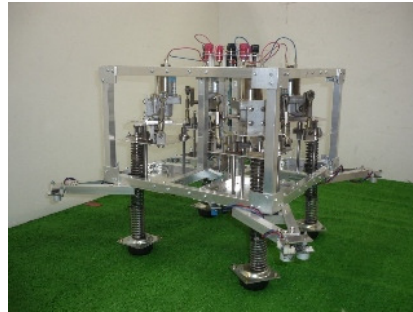
Fig. 1. Developed quadruped hopping robot
