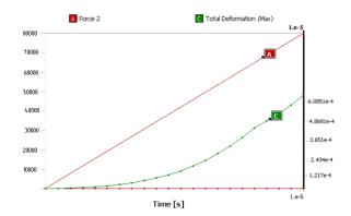
Figure 11. Result of the total deformation with respect to the applied force for the improvement design.
