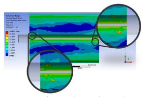
Figure 6. Contour of maximum shear stress for current design jig and fixture
