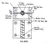
Figure 2. Concept B 'U' shape with knurling
