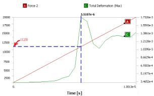
Figure 10. Result of the total deformation with respect to the applied force for the current design.
