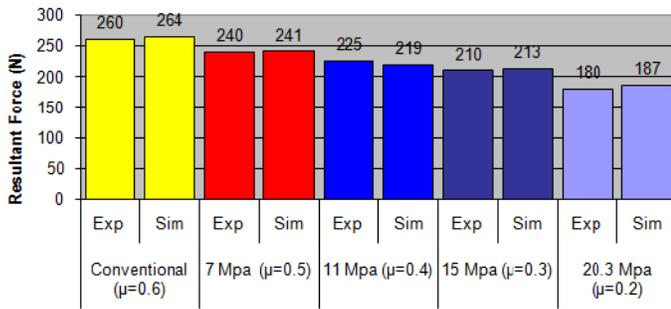
Figure 5 : Comparison of simulation and experimentally available resultant forces for different values of coolant pressure
