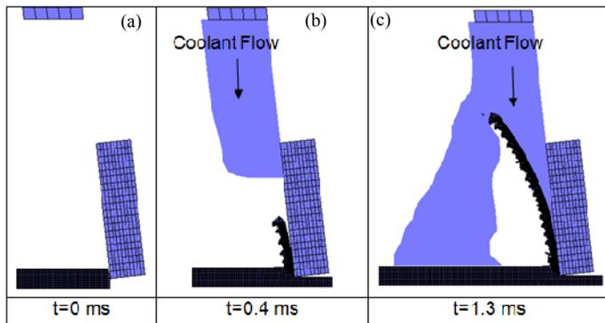
Figure 3 : Simulation of chip formation when machining with conventional coolant flow at 110 m/min cutting speed.
