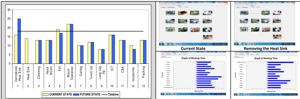
Fig. 3. Cycle time graph of main board production line
