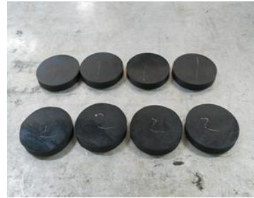
Fig. 7 Cured rubber compound for hardness test
