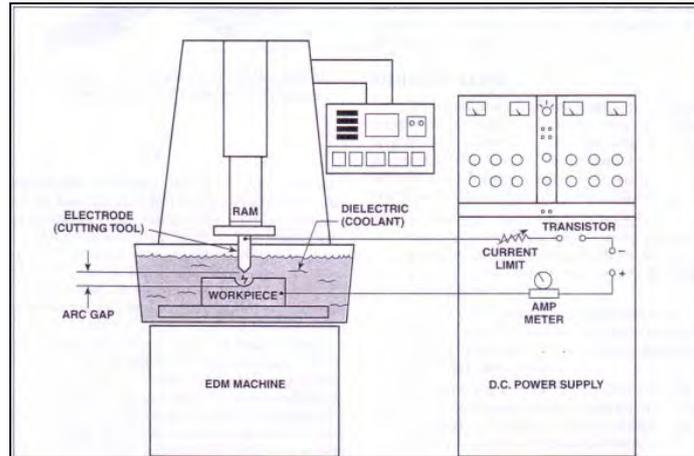
Figure 2.3: Ram-type EDMs plunge a tool, shaped to the form of the cavity required, into a workpiece (Courtesy of Kelmar Associates).
