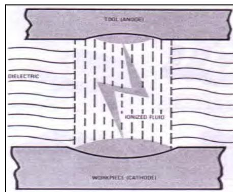
Figure 2.2: A controlled spark discharge removes a very small particle of metal during each electrical discharge (Serope *et al.* 2001).
