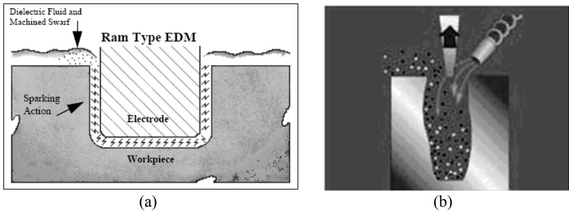
Figure 2.4: (a) Control spark removes metal during electrical discharge machine (by Technical Service Department-Brush Wellman Inc.); (b) Erosion process: ball-screw die-sinker (Zhao *et al.* 2003)
