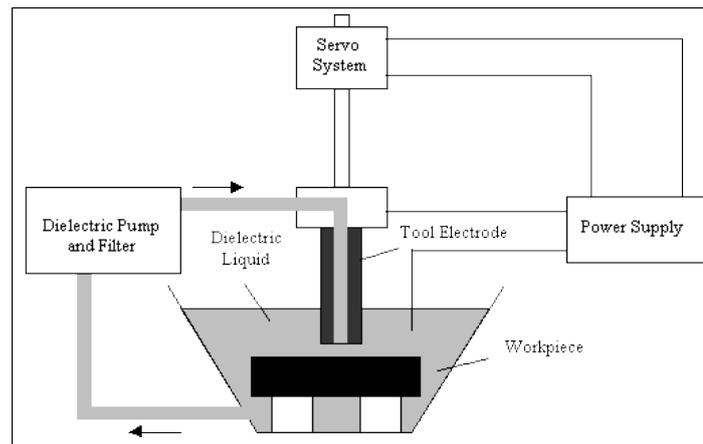
Figure 2.1: Schematic illustration of the electrical-discharge machining Process.
