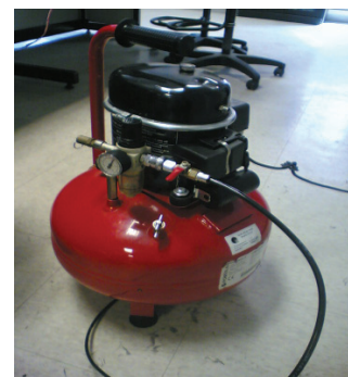
Figure 22. Mini-compressor used as pressure supplied
