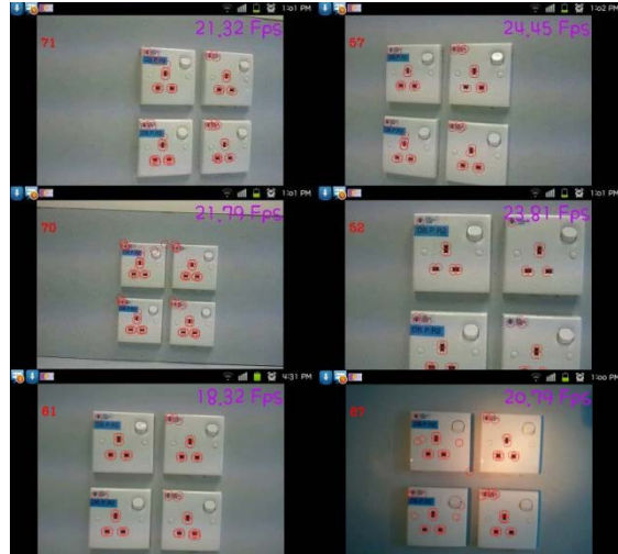
Fig. 5: From The Top Left To Top Right Are The Image With Angle Orientation For -30° And +30°, Middle Are The Images With +10 Cm And -10 Cm Distance, And Bottom, The Images With Fluorescent And Focused Incandescent Illuminations
