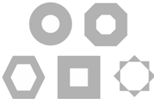
Fig. 2: Center-Surround Bi-Level Filters Approximating The Laplacian
