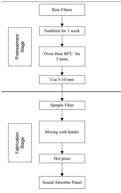
**Figure 1.** Flow chart of pre-treatment and fabrication processes.
