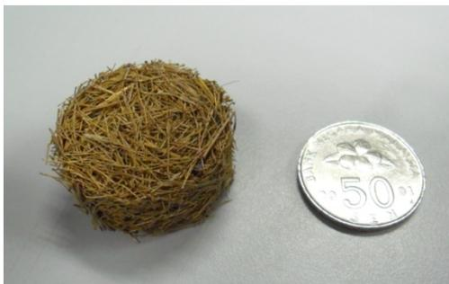
**Figure 3.** Constructed sound absorber panel
