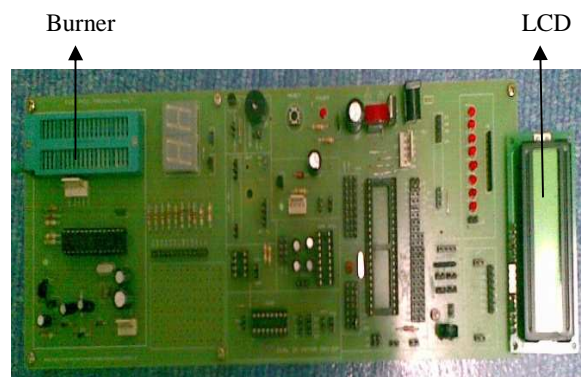
Figure 15: Circuit of controller board.
