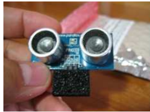
Figure 13: PING Ultrasonic Sensor Distance
