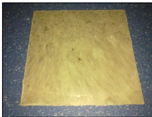
Figure 3: Specimen for dielectric testing
