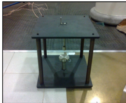
Figure 2: Electrode set-up complying with BS EN 60243-1
