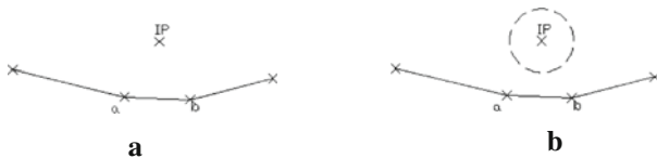
Fig. 4 a The selected edge ( a, b ) and the position of IP. b A circle is constructed with centre at IP and the radius of the circle following the empirical rule
