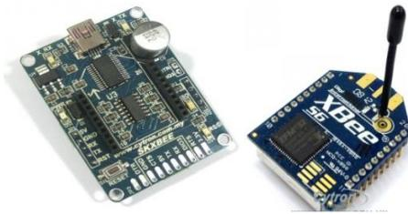
Figure 1: Xbee Module
