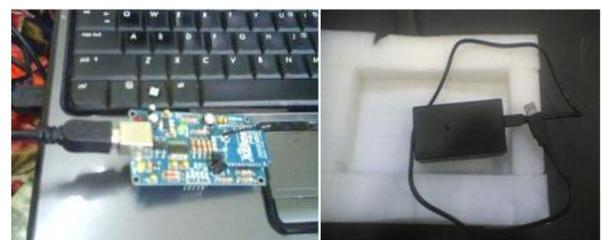
Figure 3: Connection between XBee Module and Laptop
