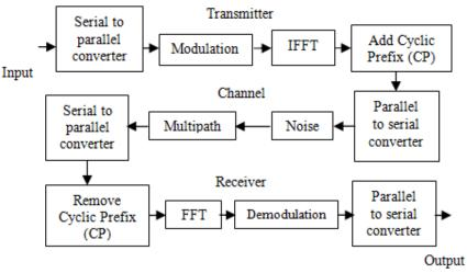
Fig. 4: OFDM Model with Cyclic Prefix
