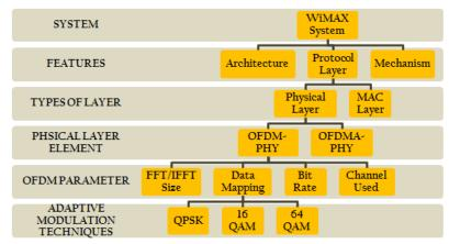
Fig. 2: Specification of WiMAX system
