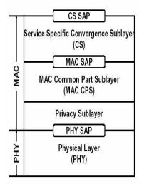
Fig. 1: WiMAX physical and MAC layer architecture
