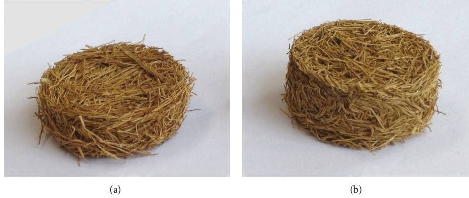
FIGURE 2: Examples of fabricated samples from paddy fibers with different thicknesses: (a) t = 10 mm, 2 grams and \rho_{\text{bulk}} = 234 \text{ kg/m}^3 and (b) t = 20 mm, 2 grams and \rho_{\text{bulk}} = 117 \text{ kg/m}^3 .
