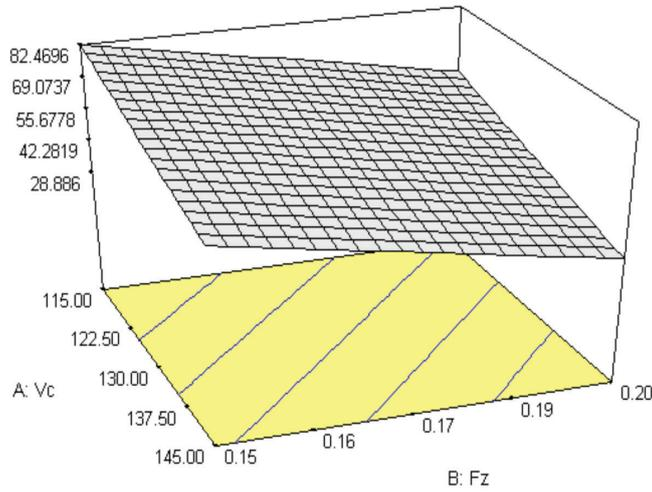
FIGURE 4. Interaction effect between cutting speed and feed rate
