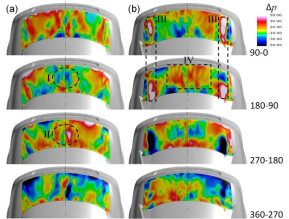
Figure 9: Trunk deck  $\Delta p$ : (a) Model A and (b) Model B.
