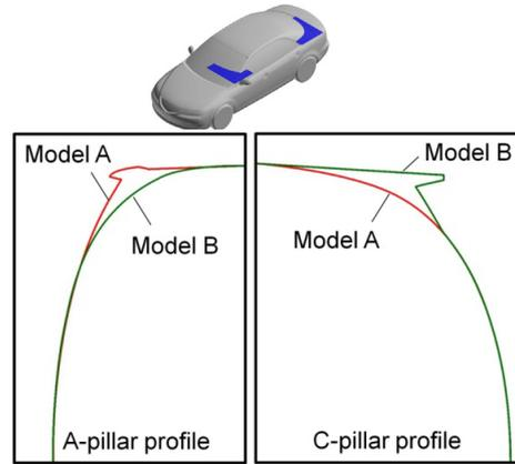
Figure 5: A- and C-pillar configurations.
