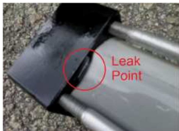
Fig.7: Leak point during the bursting leak
