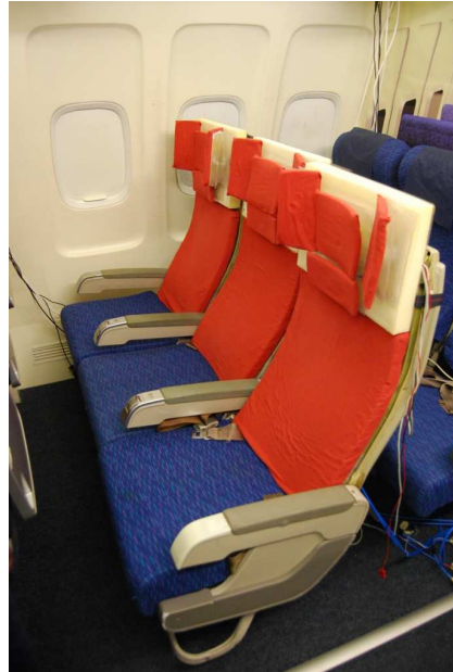
Figure 1. Three ANeSS prototypes embedded in an economy class aircraft seat
