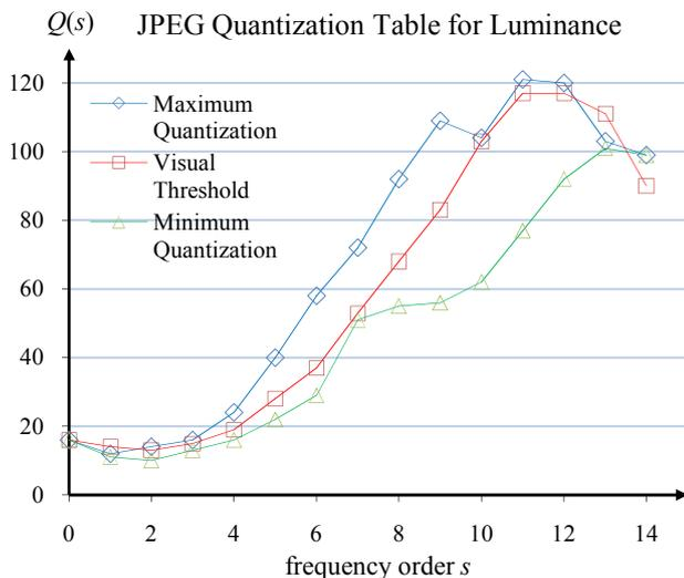
Figure 5. 2-Dimensional JPEG Quantization table for Luminance.
