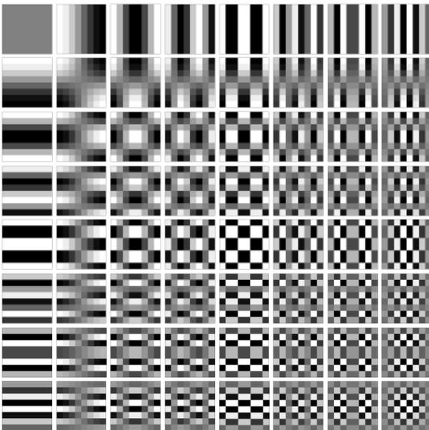
Figure 1.  $8 \times 8$  DCT basis function.
