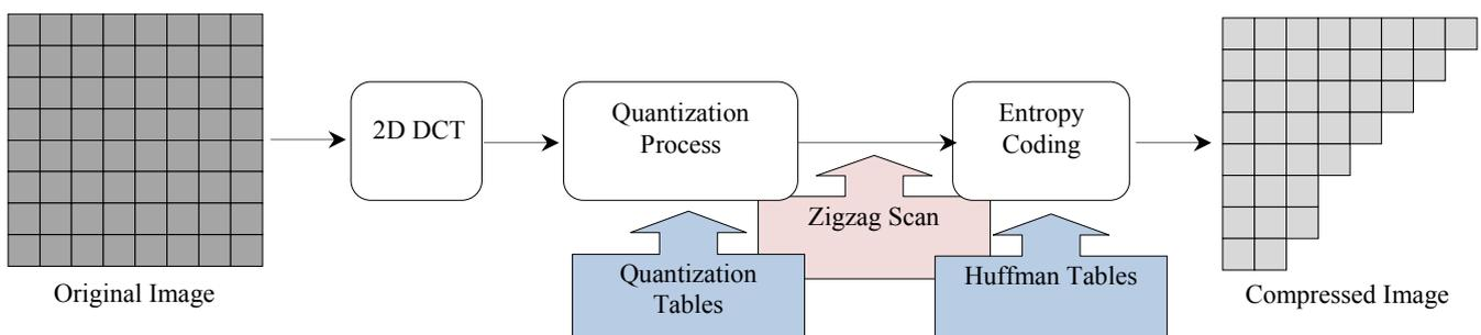
Figure 3. JPEG Image Compression consists of 2-Dimensional DCT.
