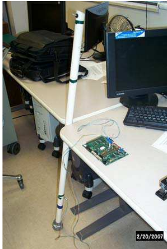
Fig -6: Walking stick prototype with gyro and Atmel EB63 evaluation board (Figure courtesy of [18]).
