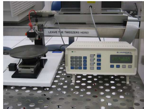
Fig. 4 : Four-point Probe for electrical conductivity measurement
