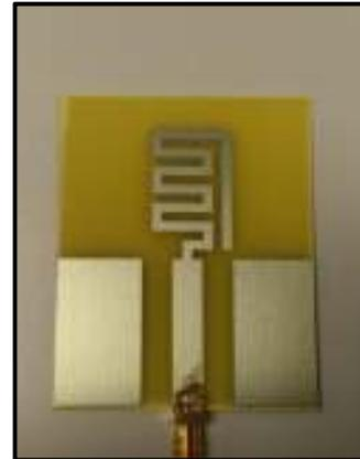
Figure 4: Antenna prototype of dual-band monopole antenna
