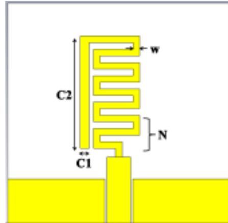
Figure 3: Geometry of the dual-band monopole antenna
